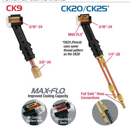
INSTALLATION: Before using this torch, tighten regulator, hose and power cable fittings with proper wrenches. Using small pliers, securely tighten all knurled hose fittings (Slide the torch handle back for access to the torch connections). Purge the regulator and TIG torch with inert gas at 20 cubic feet per hour. Following these steps will ensure contamination free welds. Repeat this procedure whenever torch or regulator fittings have been detached.
